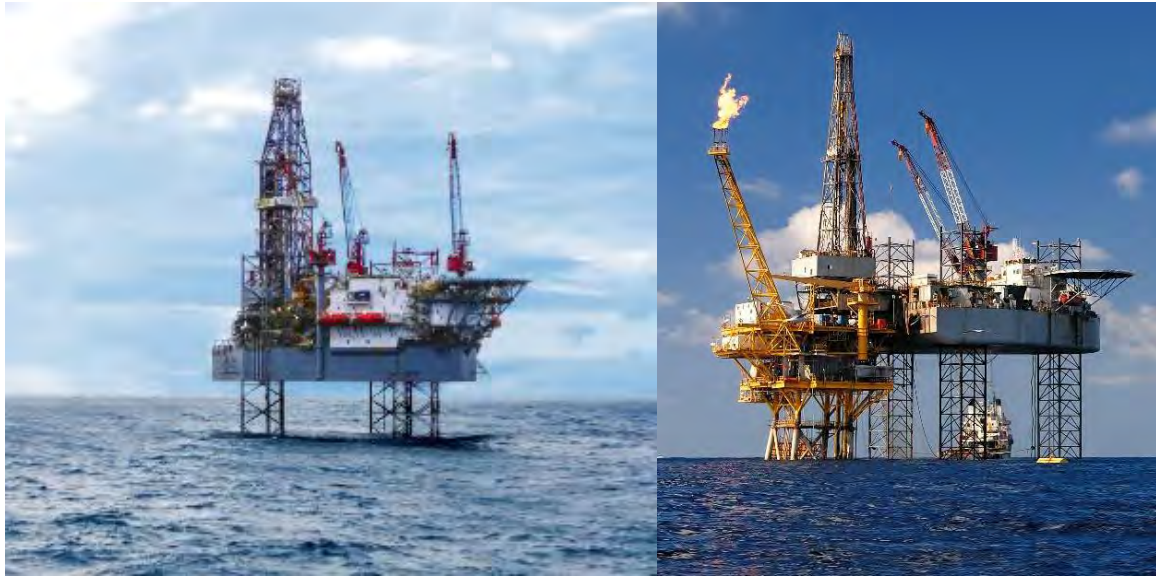
Figure 5.11 Examples of jack-up drilling rigs (in image to right, the rig is cantilevered over a small platform)
